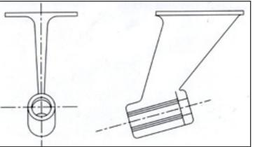
**Platform Type (vertical)** Cast in manganese or aluminium bronze and fitted with a water lubricated cutless bearing.
