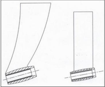
**Glass in Type.** Designed for internal bonding through GRP hulls, having the advantage of infinite adjustment during installation. Fitted with a water lubricated cutless bearing.
