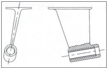
**Platform Type (angled)** Cast in manganese or aluminium bronze and fitted with a water lubricated cutless bearing.
