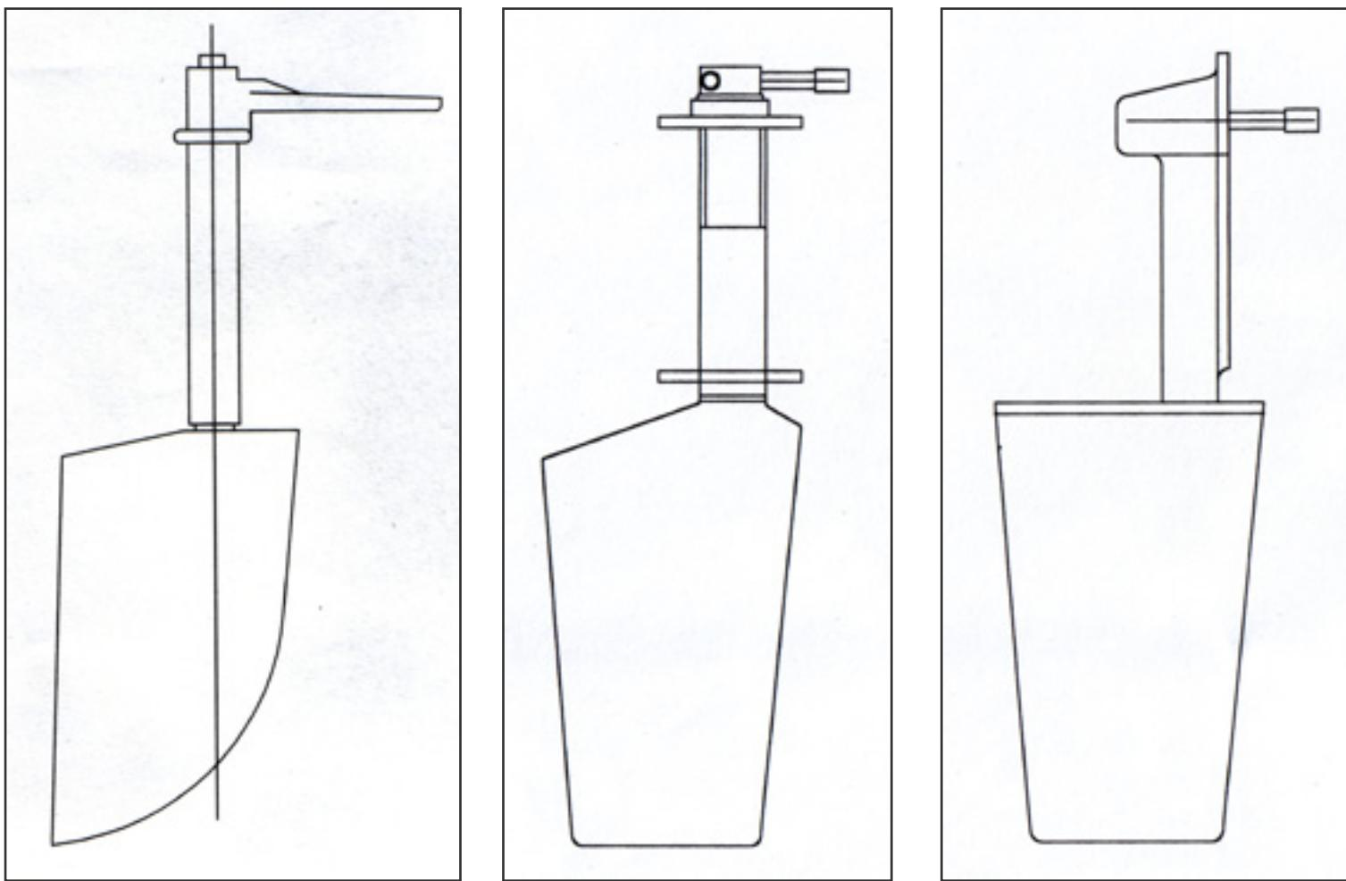
**Clements Marine** manufactures a large number of rudder profiles to suit the individual hull, ranging from slow speed displacement boats to 'deep vee' planing designs, and covering many other applications. The principal designs are shown above and include dagger type, conventional spade and wedge profile rudders.
